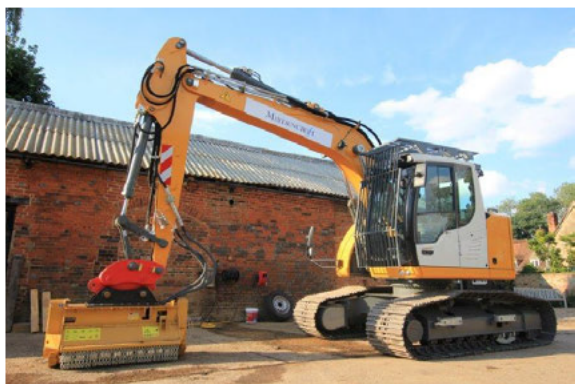
16.5 tonne caged Liebherr with Seppi Mulcher.
