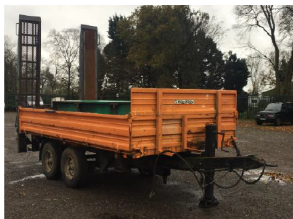
Fast-tow trailer with sides and ramps for cordwood, chip or machinery.
