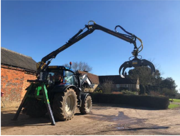
Timber grab, coupled to tractor and log trailer for on and off road collection
