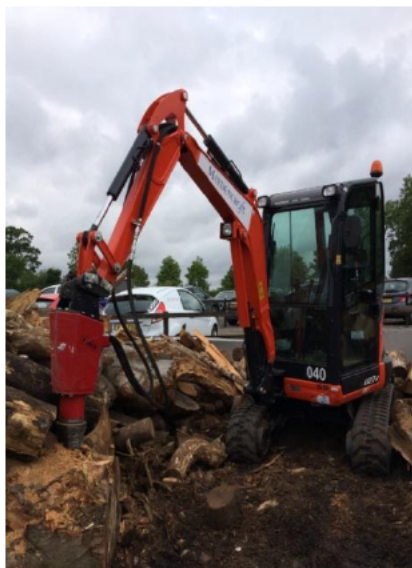
Lasco Roli 10 cone splitter in use with a Kubota.
