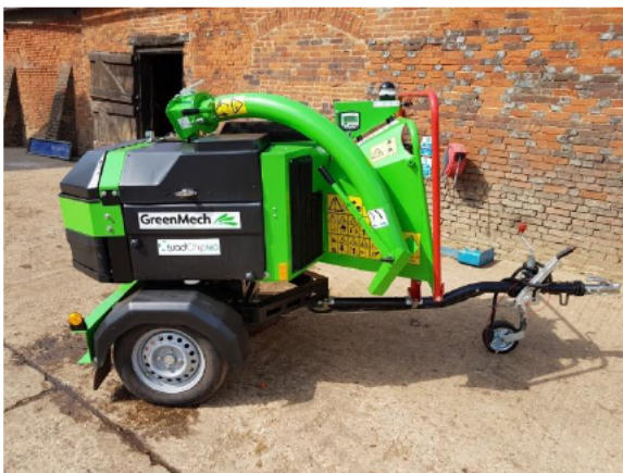
1 of 4 Turntable woodchippers for safe highway work
