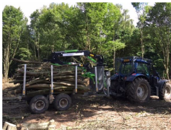
Botex 11t timber trailer with 5.7m crane and electric joysticks.
