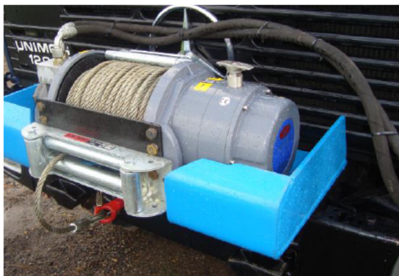
HV 15000p Hydraulic Winch mounted on a Unimog.
